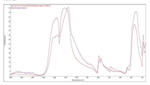
What is the difference in these two silica minerals in infrared? The neotocite is clearly SiO4 related quartz structure, with a greatly reduced 1200 cm-1 region peak. The presence of foreign cations appears linked to this band suppression, as it is consistent and does not occur otherwise.
